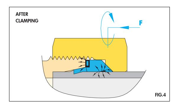
The special form of the o-ring seat is also crucial, which due to the spring effect of the ring, pre-compressed by torque **F** during clamping and thanks to the cutting shape of its rear and encloses the tube around its whole circumference (Figure 4), guaranteeing perfect tightness.
