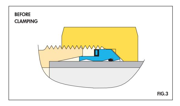
In the clamping phase, the ring AR3/C, pushed by the nut onto the 24° cone of the fitting, causes the compression of the rubber seal of the washer on the fitting, which takes the position indicated in Figure 4, making the system absolutely tight.
