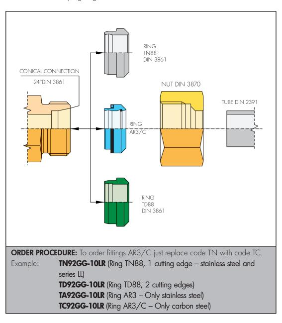
For its special characteristic of ABSOLUTE TIGHTNESS, the ring AR3/C is recommended for a use with all fittings with seals NBR (iron) or FPM (stainless steel) "SOFT SEALS", as they guarantee the same results as ring AR3/C, like absence of leakage, no oozing and externally dry tubes.
