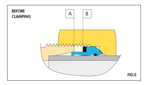
This system ensures the best cutting of the ring AR3/C into the tube. The only recommendation to follow is to check, after loosening the nut, that surfaces A and B are perfectly in contact on their whole circumference (Figure 6)
