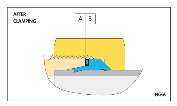
In the last clamping phase (Figure 6) the vulcanized washer has also the purpose to adjust possible off-centering caused by the addition of tolerances of the different components (BODY, TUBE, RING, NUT) compressing itself until, together with the fitting body and ring AR3/C, it becomes one complete piece.
